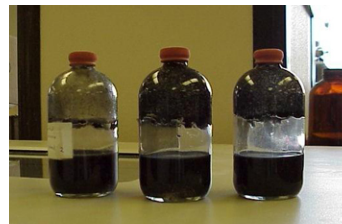
Figure 2. BMP bottles setup. Bottles are sealed to maintain a completely anaerobic environment. Source: google.com
