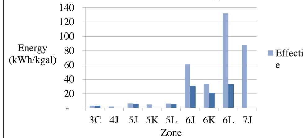
Figure 4: Comparison of Effective Embedded Energy (based on water customers receive) and Actual Embedded Energy (based on water pumped). The difference is the energy penalty due to water losses in the distribution system. It should be noted that zones 4J, 5K and 7J do not depict Actual Embedded Energy bars because of inaccurate data.
