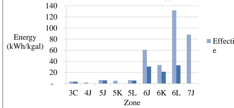
Figure 4: Comparison of Effective Embedded Energy (based on water customers receive) and Actual Embedded Energy (based on water pumped). The difference is the energy penalty due to water losses in the distribution system. It should be noted that zones 4J, 5K and 7J do not depict Actual Embedded Energy bars because of inaccurate data.
