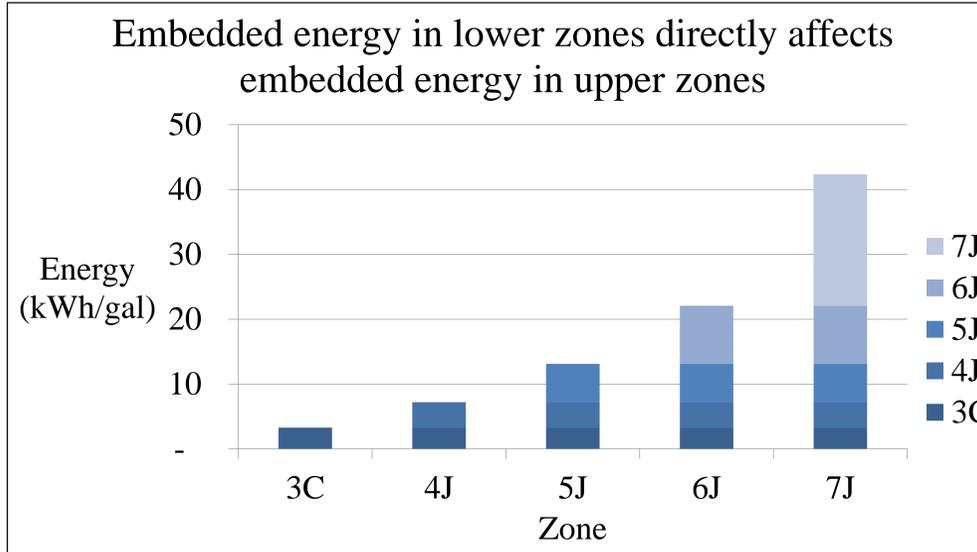
Figure 3: The embedded energy is the amount of energy traveling throughout the system. Higher zones, which are at higher elevations, further down the system chains have cumulative embedded energy in the water.
