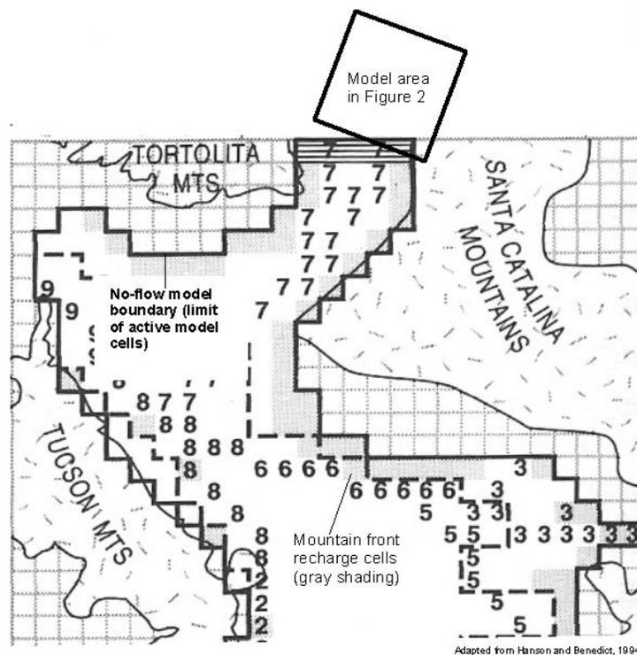
Figure 1. Model domain for northern part of Tucson Active Management Area model, showing 1 x 1 mile cell size, mountain front recharge cells, and location of model shown in Figure 2.
