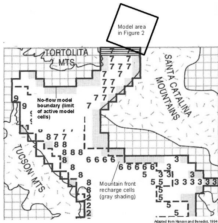
Figure 1. Model domain for northern part of Tucson Active Management Area model, showing 1 x 1 mile cell size, mountain front recharge cells, and location of model shown in Figure 2.
