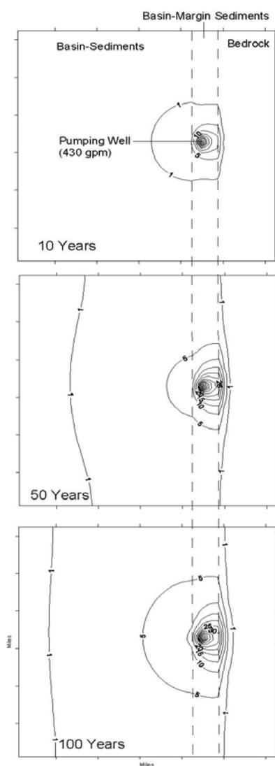
**Figure 4.** Simulated groundwater drawdown contours, in feet, from a single pumping well after 10, 50, and 100 years (dashed vertical lines show boundary of hydrogeological units).
